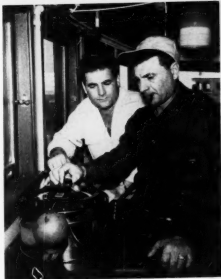
Navigator Louis Sitta, left, and Capt. Sal Alioto of the tuna clipper Commander , operating the new Sperry magnetic compass pilot recently installed in the vessel at San Diego. This single unit, with a Kelvin-White 8-inch compass and a controller mounted on top, operates with the steering engine. Captain Alioto has his hand on the knob by which the course is set. Commander was built by Birchfield Boiler, Tacoma, and is owned by Al Davies.
